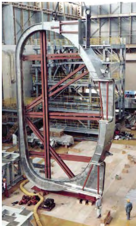
Testing, testing. Engineers have already built pieces of ITER, such as this slice of vacuum vessel, to test construction.
